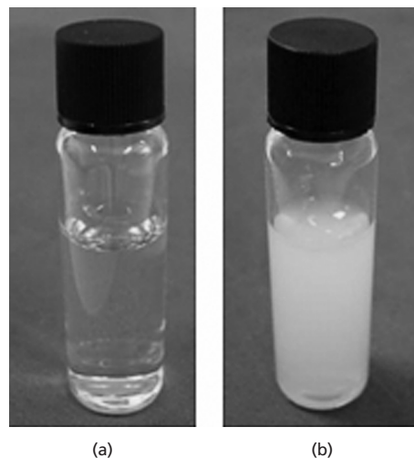
Figure 1 Solution of a temperature-responsive polymer below (a) and above (b) the temperature of phase separation (TPS).
